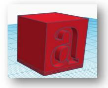
1. Drag and drop the **Box** onto the **Workplane**. The box will already have dimensions of 20 mm x 20 mm x 20 mm. (Keep these dimensions)
