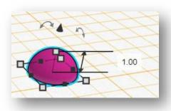
4. Move your braille dot to the top left part of your box. Click the **Duplicate** button. Click and hold on the braille dot, the new copy is right on top. Hold **Shift** on the keyboard and drag the dot until it reads 5 mm away from the first dot.
