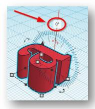
6. Position the letter to be on a side of the box. Use the **black cone** to move the letter up and down.
