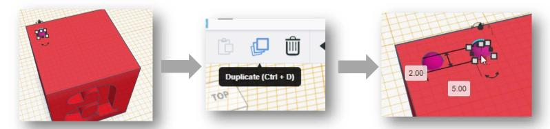
5. Select both dots by selecting one, holding **Shift** and selecting the second dot. Select **Duplicate**. While holding **Shift**, click and drag one of the dots (2 dots will move) 5 mm down. Right after you move the dots, both of the new dots will be highlighted. Click on the **Duplicate** button again, this will make a 3<sup>rd</sup> row of dots.
