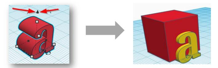
7. Select both shapes by clicking on one shape, hold shift, and select the second shape. At the top right where the color of the shape is, it will show that two shapes are selected, **Shapes(2)**. Click the **Align** button ( ), and click on both of the highlight dots below. This will center the letter onto your box.
