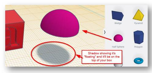
3. Resize the half sphere using the handles. The length and width needs to be 2 mm each and the height is 1 mm.
